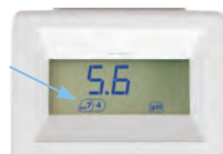
Successful pH 7 and pH 4 calibration
