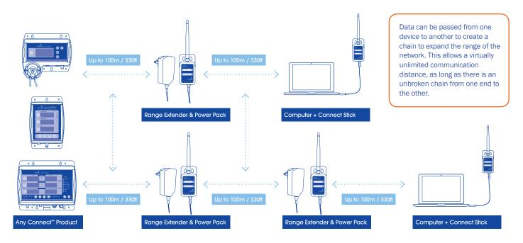
If the distance between two devices is too far for a wireless link to be formed, a Bluelab® Connect™ Range Extender 2 can be placed between them. This effectively doubles communication distance.
